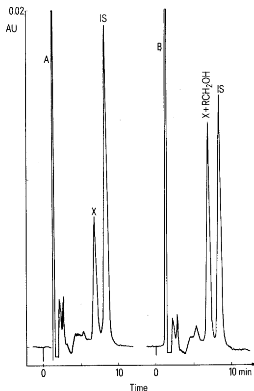
Fig. 2. Chromatogram of a corpus luteum extract (A) and of the supplemented corpus luteum extract (with 50 ng retinol) (B). Conditions: same as figure 1 except mobile phase, n-hexane/ \text{CH}_2\text{Cl}_2 /isopropanol (200/50/1.75); flow, 0.25 ml/min. Peak identity: endogenous retinol (X), internal standard (IS) and endogenous retinol + supplemented retinol ( \text{X} + \text{RCH}_2\text{OH} ).
